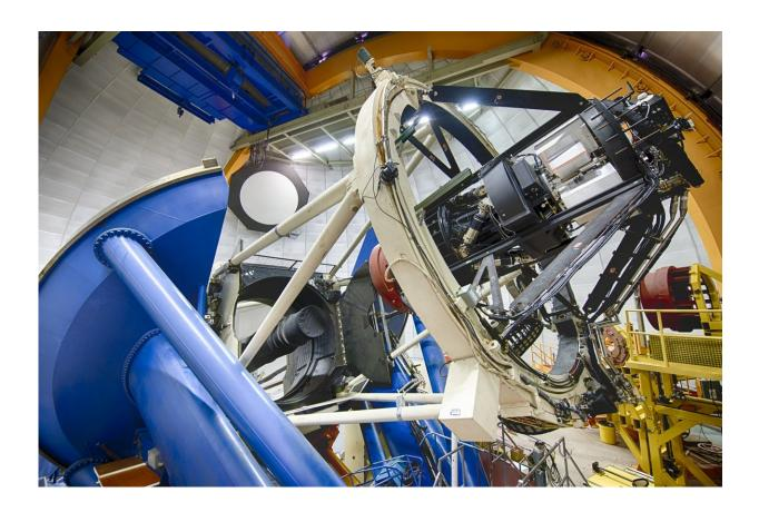
The Dark Energy Camera is mounted on the 4-meter Blanco telescope at the Cerro Tololo Inter-American Observatory in Chile. The final day of data-taking for the Dark Energy Survey is Jan. 9. Credit: Fermilab
