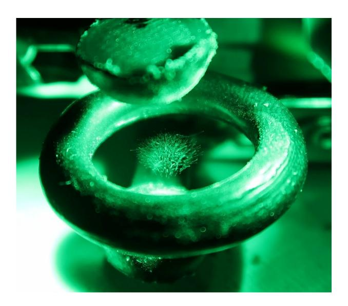
Electrically charged particles suspended in a 3-D-printed particle trap. Credit: Janna Zoe Vischer/Julia Woithe/CERN
