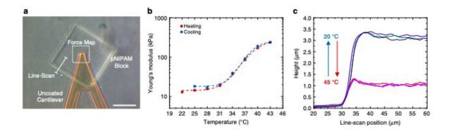
Mechanical analysis of a pNIPAM block fabricated by 3D laser lithography. a) Optical micrograph in the AFM with overlayed indications for the force measurements and the line-scan. Scale bar is 50  $\mu$ m. b) Measured Young's Modulus as a function of temperature for a stepwise heating and cooling of the sample. c) Height measurement via line-scanning from the glass substrate on top of the pNIPAM block. The different colors depict several cycles of heating and cooling. Credit: Hippler et al.
