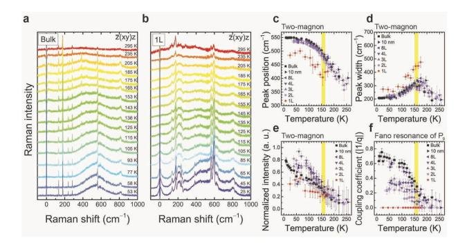
Figure 2: The comparison between bulk and monolayer NiPS3 at different temperatures. Bulk (a) and monolayer (b) NiPS3 reveal a different signature in the Raman spectra. The big peak at around 550 cm-1 in the one-atom thick sample is a sign that the magnetic ordering is lost. Credit: Institute for Basic Science
