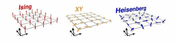
Figure 1: Spins at play. Electrons' spins in different materials might be constrained in certain orientations. The Ising model deals with spins which are pointing either up or down. The XY model explains the behavior of materials where the spins are free to move only on the x and y axis, and the Heisenberg model is about spins that point in any direction, much like clock hands. Credit: Institute for Basic Science
