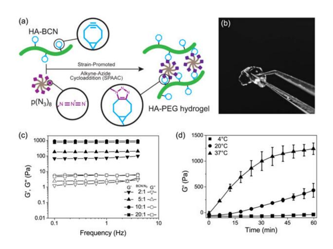
(a) Schematic representation of the formation of HA-PEG hydrogels through a strain-promoted alkyne-azide cycloaddition reaction. (b) Photograph of a HA-PEG hydrogel after formation. (c) Frequency sweeps of HA-PEG hydrogels with different BCN to N3 ratios. (d) Gelation time experiment showing the increase of G' over time during gelation of HA-PEG hydrogels (10:1 BCN:N3) at different temperatures. Credit: *Biofabrication*, doi:
