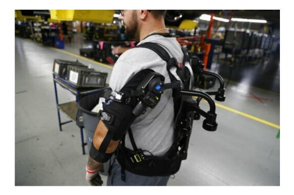
In this Sept. 18, 2018, photo Ford assembly line worker Nicholas Gotts wears a new wearable technology called an EksoVest in Flat Rock, Mich. The wearable device, that the automaker will be providing plants around the world, provides lift assistance from 5 to 15 pounds per arm. (AP Photo/Carlos Osorio)
