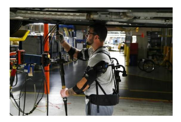
In this Sept. 18, 2018, photo Ford assembly line worker Nicholas Gotts, wearing a new wearable technology called an EksoVest, works on a vehicle in Flat Rock, Mich. The wearable device, that the automaker will be providing plants around the world, provides lift assistance from 5 to 15 pounds per arm. (AP Photo/Carlos Osorio)
