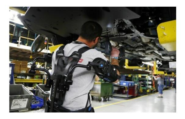
In this Sept. 18, 2018, photo Ford assembly line worker Nicholas Gotts, wearing a new wearable technology called an EksoVest, works on a vehicle in Flat Rock, Mich. The wearable device, that the automaker will be providing plants around the world, provides lift assistance from 5 to 15 pounds per arm. (AP
