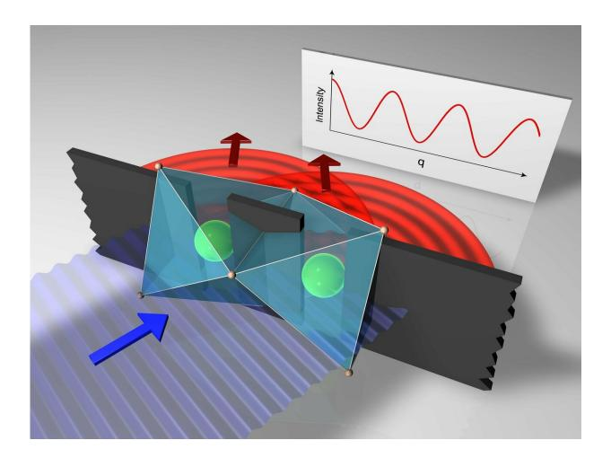
An intense beam of high-energy X-ray photons (violet) hits two adjacent iridium atoms (green) in the crystal. This excites electrons in the atoms for a short time. The atoms emit X-ray photons which overlap behind the two iridium atoms (red) and can be analyzed as interference images. Credit: Markus Grueninger, University of Cologne
