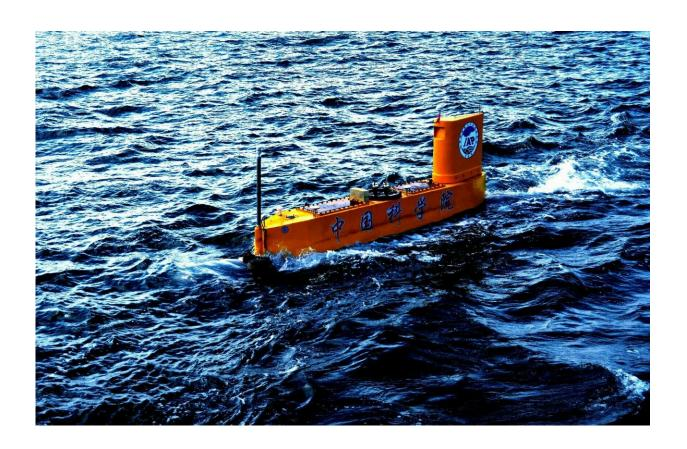
An unmanned semi-submersible vehicle (USSV) developed by Chinese Academy of Sciences. The photo was taken at the first USSV sea trial in Bohai Bay on 13 June 2017. Credit: Siping Zheng
