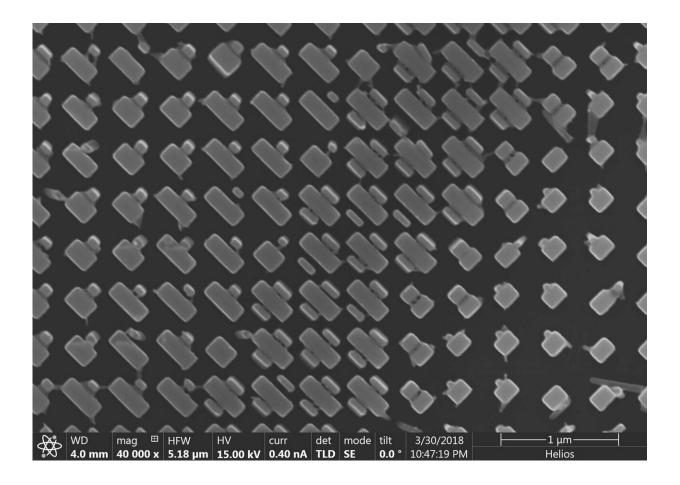
These newly designed nano-structures on the surface of a metalens can focus light regardless of its polarization, doubling the efficiency of the lens. Credit: Capasso Lab/Harvard SEAS
