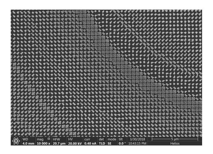
These newly designed nano-structures on the surface of a metalens can focus light regardless of its polarization, doubling the efficiency of the lens. Credit: Capasso Lab/Harvard SEAS
