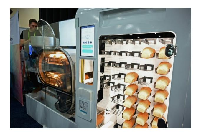
The BreadBot—a fully automated bread-making machine that mixes, kneads, proofs, bakes and sells bread like a vending machine is displayed at CES Unveiled, the preview event for the 2019 Consumer Electronics Show
