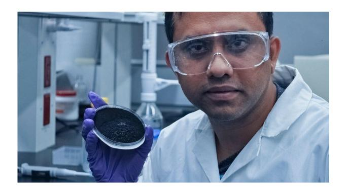
Samrat Alam holds a sample of biochar. Alam and U of A geochemist Daniel Alessi found that the inexpensive charcoal can be tailored for specific uses like water treatment or soil remediation by controlling the temperature and organic material used to produce it. Credit: Samrat Alam
