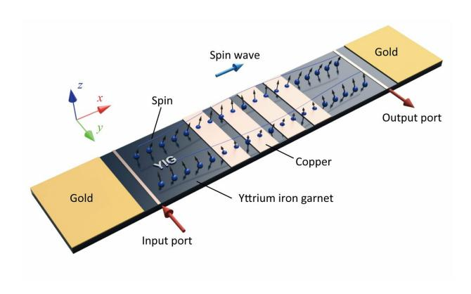
A model of a spin wave device realized by combining yttrium iron garnet, gold and copper. 'Stop band,' which does not allow spin waves of specific frequencies to pass, were exhibited. Credit: Toyohashi University of Technology
