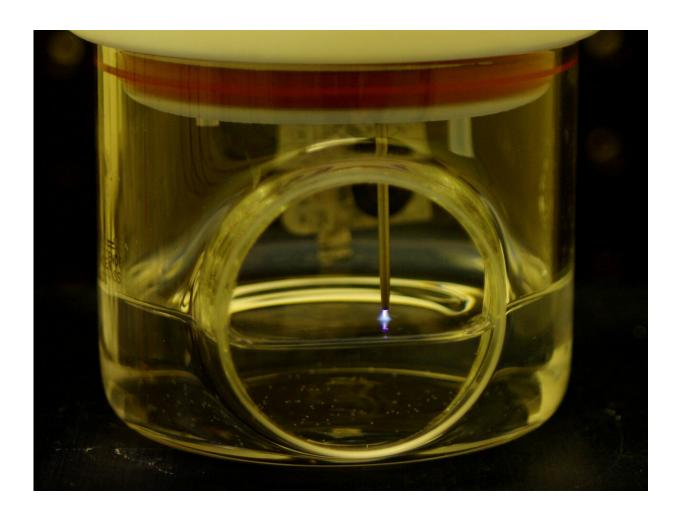
Graphic illustration showing protonated water reacting with nitrogen molecules to form ammonia at a plasma-liquid interface. Credit: Case Western Reserve University
