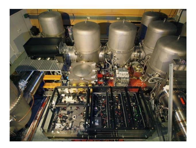
The GEO600 squeezed light source (in the foreground) inside the GEO600 clean room together with the vacuum tanks (in the background).. Credit: H.Grote/Max Planck Institute for Gravitational Physics
