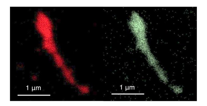
Energy dispersive X-ray spectroscopy images of the sample of a solution with virus. Color coding of atomic species: germanium, red; tin, green. Credit: SUTD
