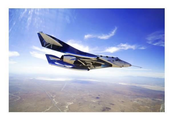
This May 29, 2018 photo provided by Virgin Galactic shows the VSS Unity craft during a supersonic flight test. The spaceship isn't launched from the ground but is carried beneath a special aircraft to an altitude around 50,000 feet (15,240 meters). There, it's released before igniting its rocket engine and climbing. (Virgin Galactic via AP)
