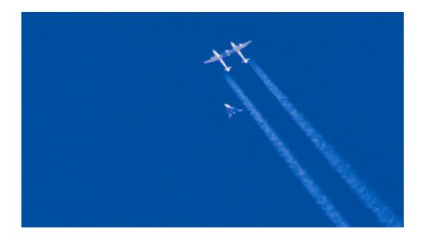
In this Jan. 11, 2018 photo provided by Virgin Galactic, the VSS Unity is released from the WhiteKnightTwo aircraft during a gliding test for SpaceShipTwo near Mojave, Calif. The spaceship isn't launched from the ground but is carried beneath the special aircraft to an altitude around 50,000 feet (15,240 meters). There, it's released before igniting its rocket engine and climbing. (Virgin Galactic via AP)
