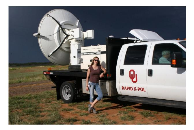
Jana Houser standing next to the Rapid X-Pol radar instrument, a new type of rapidly-scanning mobile radar system, during a storm chase on 8 May 2012. Credit: Jana Houser.
