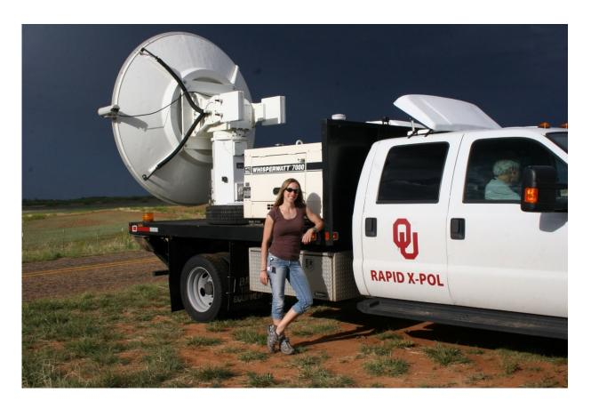
Jana Houser standing next to the Rapid X-Pol radar instrument, a new type of rapidly-scanning mobile radar system, during a storm chase on 8 May 2012. Credit: Jana Houser.
