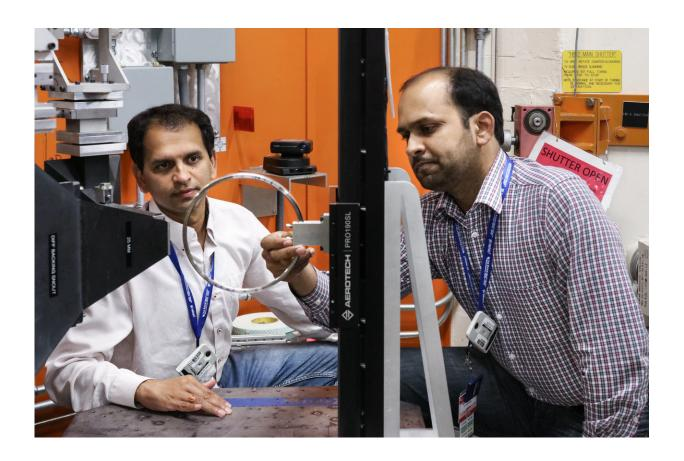
Timken researchers Vikram Bedekar (left) and Rohit Voothaluru are aiming to improve bearing manufacturing processes by using neutrons at HFIR's HB-2B. Credit: ORNL/Genevieve Martin
