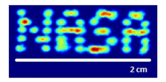
This image demonstrates the control that the Goddard-AOSense team has over the paths of atoms. In this demonstration, they manipulated the path to form the acronym, NASA. Credit: AOSense, Inc.
