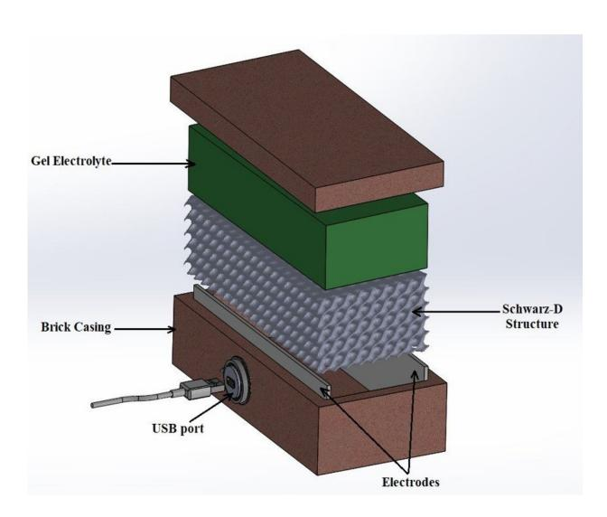
An international team of scientists, led by King's College London, have developed a thermogalvanic brick that generates electricity as long as the two faces of the brick are at different temperatures. Credit: King's College London
