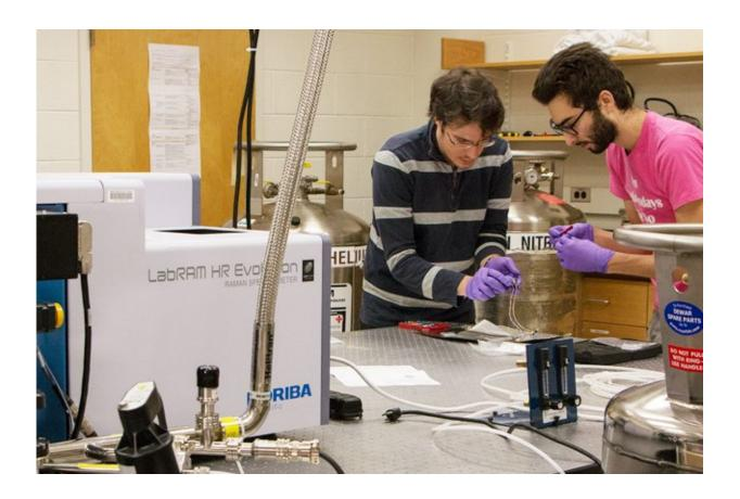
Riccardo Comin (left), an assistant professor of physics, and physics graduate student Abraham Levitan assemble the contacts on a sample holder that they'll use to study the effects of high current on the superconducting material yttrium barium copper oxide, in the cryogenic optical spectrometer seen in the foreground. The setup enables the researchers to perform Raman spectroscopy down to 4 kelvins under a voltage, or current, bias. Credit: Denis Paiste/Materials Research Laboratory
