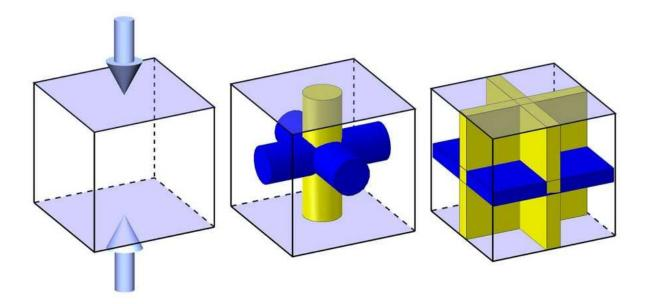
When it comes to withstanding loads in all three dimensions (from above or below, left or right, and back or front), plate-lattices have a clear advantage over truss-lattices. The following thought experiment helps in understanding this: Imagine two cubes with very thin outside walls. Inside them are struts to prevent the cubes being compressed when external pressure is applied. One cube uses
