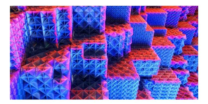
Plate-lattices will be the design of choice for future lightweight porous materials. Credit: ETH Zurich / Marc Day
