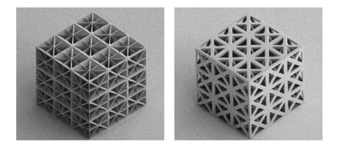
Example of additively-manufactured polymer plate-lattice (left) and a trusslattice (right). The cube on the left is constructed from plates measuring just 2 micrometres in thickness. Both cubes have an edge length of 0.2 millimetres. Credit: Tancogne-Dejean T et al. Advanced Materials 2018
