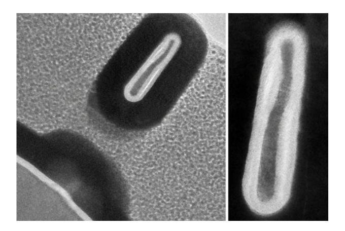
Using a new manufacturing technique, MIT researchers fabricated a 3-D transistor less than half the width of today's slimmest commercial models, which could help cram far more transistors onto a single computer chip. Pictured is a cross-section of one of the researchers' transistors that measures only 3 nanometers wide. Credit: Massachusetts Institute of Technology
