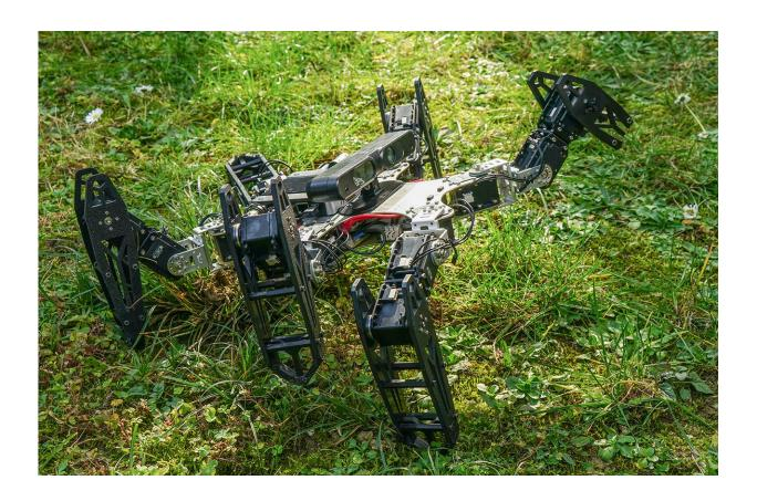
In trials, the ResiBot robot learned to walk again in less than two minutes after one of its legs was removed. Credit: Antoine Cully / Sorbonne University
