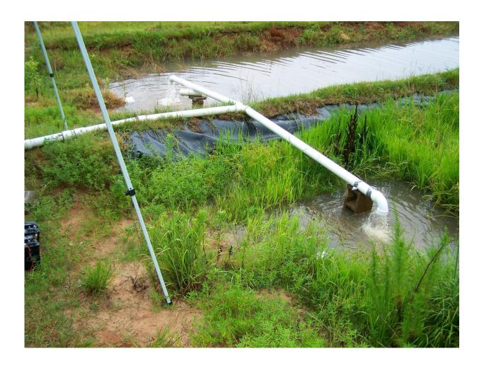
A delivery system applies a simulated storm runoff containing pesticides and water to rice and control (bare) systems. Credit: Matt Moore
