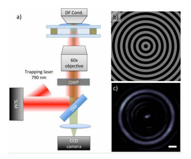
Diagram of the experimental optical trap described in the text. The setup contains a spatial light modulator (SLM), dark field condenser (DF Cond.), dichroic-mirror (DM) and quarter wave plate (QWP). The trapping laser is reflected from the SLM, which is used for beam shaping. Dark-field illumination that scatters from the Ag (silver) nanoparticles is collected by the
