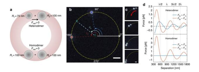
A schematic diagram of the experiment: a) Example trajectories for a homodimer (black) and a heterodimer (color) that are moving in counterclockwise (green) and clockwise (blue) directions. Distribution of instantaneous angular velocities (gray dots) and the mean angular velocities of the homodimers (b, black) and heterodimers (c, orange) as a function of interparticle separation. The bin size is 300 nm. The mean angular velocity value
