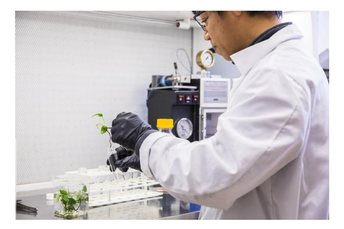
Long Zhang, a research scientist in the UW's civil and environmental engineering department, puts a pothos ivy plant into a glass tube to test its ability to break down benzene or chloroform. Credit: Mark Stone/University of Washington
