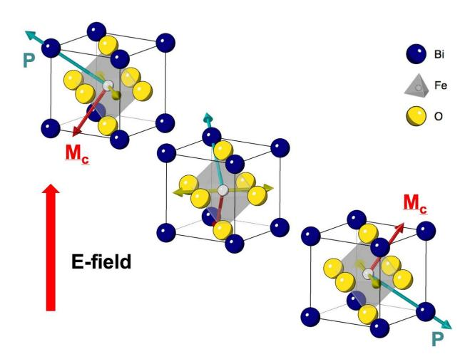
MESO devices, based on magneto-electric and spin-orbit materials, could someday replace the ubiquitous semiconductor transistor, today represented by CMOS. MESO uses up-and-down magnetic spin states in a multiferroic material to store binary information and conduct logic operations. Credit: Intel graphic
