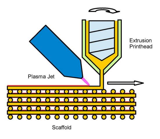
How to manufacture coated scaffolds: Immediately after extrusion, the scaffold structures are treated with a cold plasma. Credit: Fraunhofer IST
