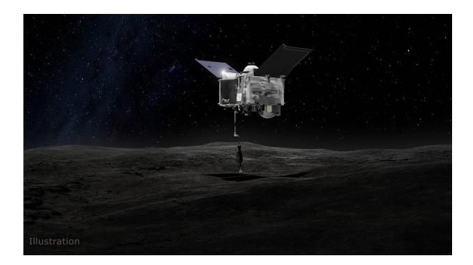
This artist's concept shows the Origins Spectral Interpretation Resource Identification Security - Regolith Explorer (OSIRIS-REx) spacecraft contacting the asteroid Bennu with the Touch-And-Go Sample Arm Mechanism or TAGSAM. The mission aims to return a sample of Bennu's surface coating to Earth for study as well as return detailed information about the asteroid and it's trajectory. Credit: NASA's Goddard Space Flight Center
