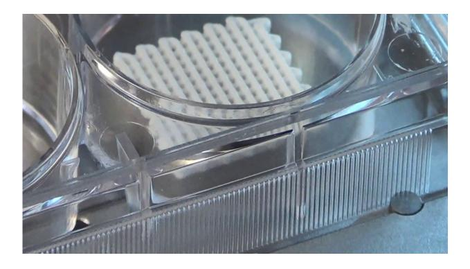
The 3D bioprinter platform can create 3D scaffolds in the lab using polymers to engineer layer-by-layer biomimetic architecture. Image: https://goo.gl/images/xp1ADW Credit: Biomedical Materials, doi: 10.1088/1748-605x/aaeb82
