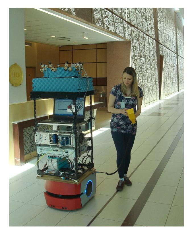
NIST researcher Jelena Senic drives a robot used to measure the performance of different antenna beam patterns. The mobile platform enables researchers to
