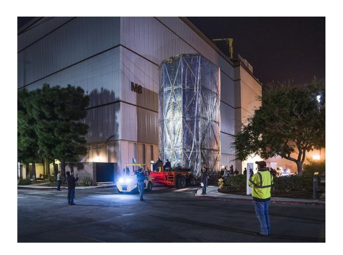
In this photo, the big silvery-looking box is the mobile clean room, which project personnel call the "In-Plant Transporter." Nestled inside and visible through the translucent wrapping of the In-Plant Transporter is the Webb flight spacecraft element, which is the assembly of the spacecraft bus and sunshield. Here, the spacecraft element was being moved from the clean room where it was constructed to another building where it will undergo vibration and thermal-
