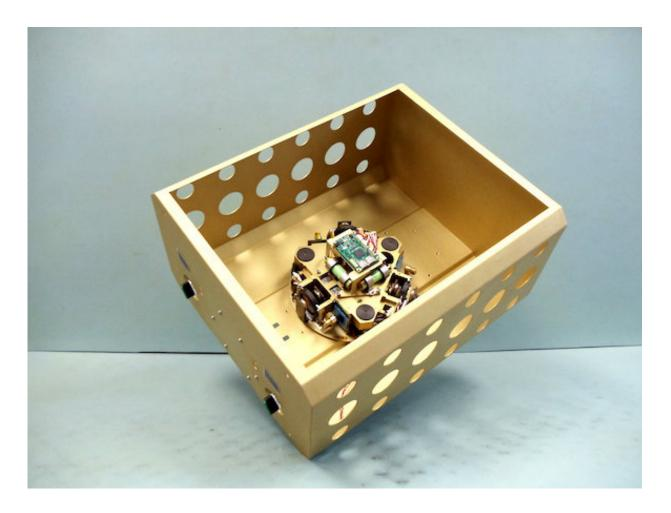
The Vibration Isolation Platform from Controlled Dynamics Inc. has completed five successful Flight Opportunities-sponsored flights on suborbital reusable launch vehicles (sRLVs). The scheduled flight on SpaceShipTwo will mark its sixth. Credit: Controlled Dynamics Inc.
