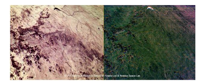
False color images of desert highland in southern Sahara. The image on the left depicts the changes of the soil type across the image while the image on the right displays changes in soil moisture. The water reservoir in the upper part of the image is very well highlighted in this image, when compared to the dark rocks. Credit: VTT Technical Research Centre of Finland
