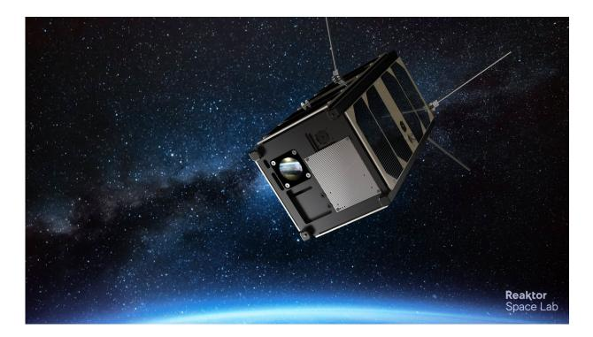
3-D render of the Reaktor Hello World satellite hosting the first ever miniature infrared hyperspectral imager for satellites. The satellite is only 10 centimeters wide and 20 centimeters long. Credit: VTT Technical Research Centre of Finland
