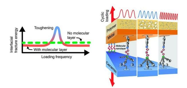
Illustrations of frequency-dependent toughening in a polymer-metal-nanoglueceramic composite. Credit: Rensselaer Polytechnic Institute
