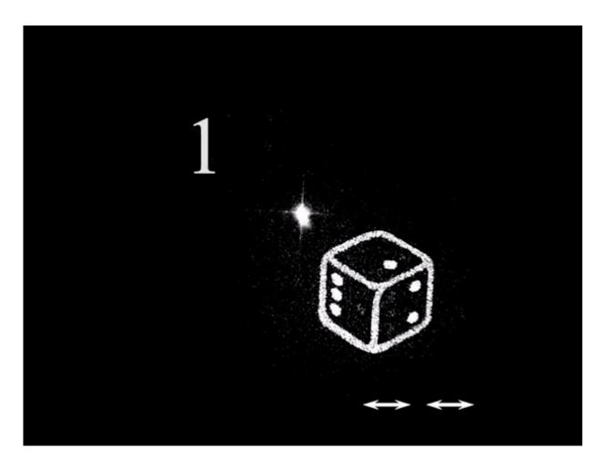
Multichannel polarization-multiplexed holograms ("Dice"). Credit: Light: Science & Applications, doi: 10.1038/s41377-018-0091-0.
