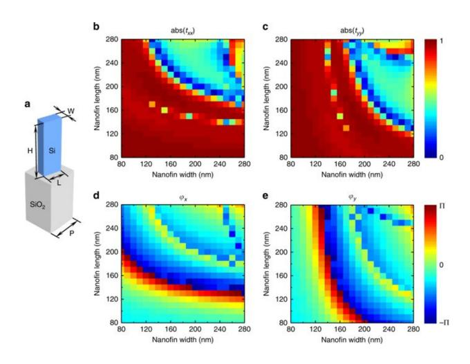
a) Schematic illustration of an amorphous silicon nanofin positioned on a glass substrate. The metasurface will be composed of a periodic arrangement of such unit-cells. b—e) Simulation results for the amplitude and phase of the transmission coefficients txx and tyy shown for a 2D parameter optimization by using a rigorous coupled wave analysis method. The length and width of the
