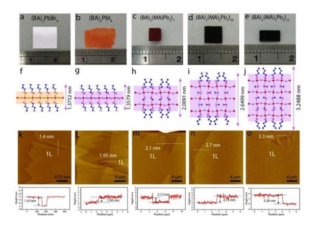
Figure 1: (a - e) Optical image of large sized 2D hybrid perovskites (single crystal) and different homologous series (compounds with the same functional group but differ by the number of repeating units) from n = 1 to n = 4. (f - j) Schematics showing the structure of the unit cell. (k - o) Atomic force microscopy images and profile of the exfoliated single unit cell perovskite layers. Credit: National University of Singapore
