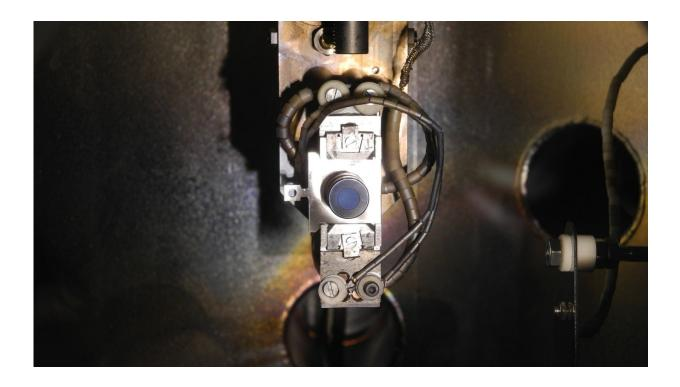
Photocathode after its production in the preparatory system. Credit: HZB
