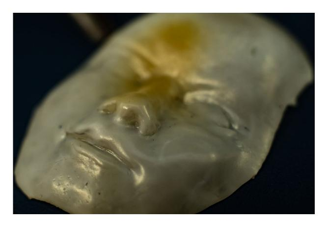
A face made of a unique polymer at Rice University takes shape when cooled and flattens when heated. The material may be useful in the creation of soft robots and for biomedical applications. Credit: Jeff Fitlow/Rice University
