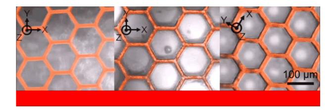
Liquid crystal elastomers deform in response to heat, and the shape they take depends on the alignment of their internal crystalline elements, which can be determined by exposing them to different magnetic fields during formation. Credit: Wyss Institute at Harvard University
