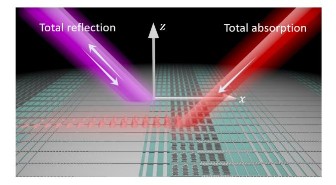
The team from Aalto use gradient metasurfaces to engineer the contrast ratio of brightness for waves coming from two oppositely tilted angles. Credit: Xuchen Wang/Aalto University
