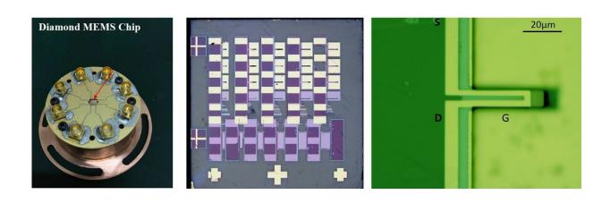
Micrographs of the diamond MEMS chip developed through this research and one of the diamond cantilevers integrated into the chip Credit: NIMS
