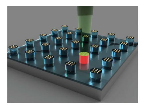
Laser-induced heating of nanoparticles on micropillars for carbon nanotube growth. Credit: Northwestern University
