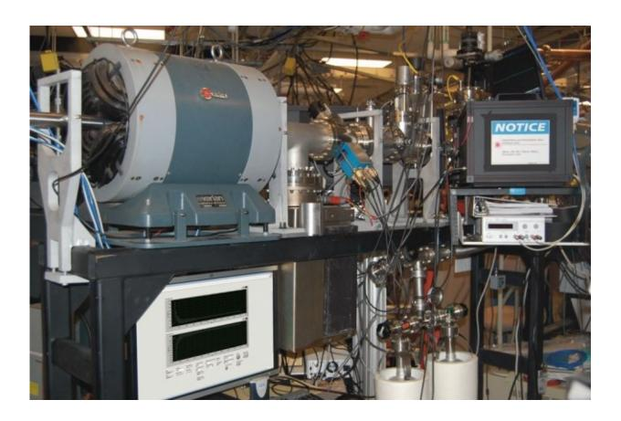
The ion beamline at Sandia National Labs where the new radiation damage measurement system has been installed and tested. The radiation damage process is observed in a target chamber located behind the black-box laser enclosure on the right of the image. Credit: Cody Dennett
