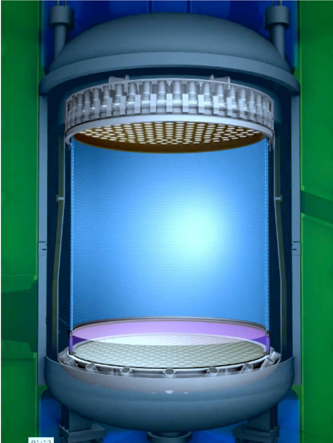
This rendering shows a cutaway view of the LZ xenon tank (center), with PMT arrays at the top and bottom of the tank. Credit: Greg Stewart/SLAC National Accelerator Laboratory
