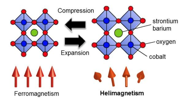
Figure: Schematic illustration of the helimagnetic-ferromagnetic transition driven by the lattice expansion/compression in the cubic perovskite Sr1-xBaxCoO3. Credit: S. Ishiwata and H. Sakai
