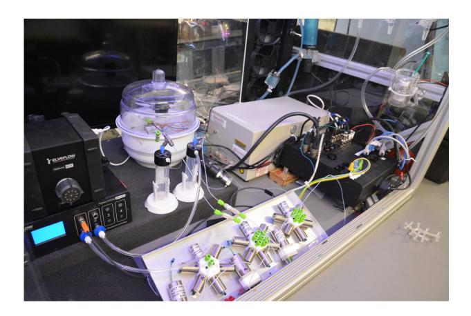
Thanks to a National Science Foundation grant, NYU Tandon School of Engineering students built the world's first artificially intelligent microreactor. The equipment allows scientists to study reactions using just a few drops of fluid instead of perhaps 100 liters of chemicals, thereby preventing chemical waste and saving considerable energy. Credit: NYU Tandon
