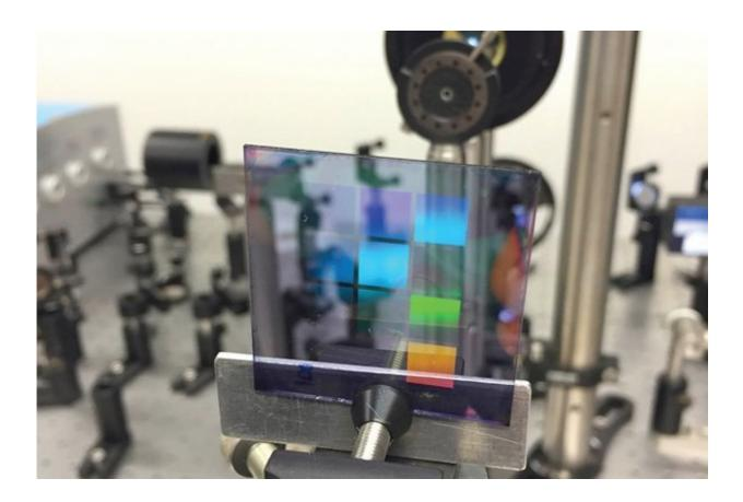
An experimental sample of the new laser. It contains ten patches that each have their own silver nanoparticle pattern. The colors on the sample are not the laser light (the laser is not on) but reflections, similar to the colors that can be seen on the surface of a compact disk. Credit: Alexei Halpin, Eindhoven University of Technology
