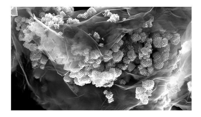
HRSEM picture of a 2D/3D nanocomposite based on graphene. Credit: Freddy Kleitz/Universität Wien; Glaudio Gerbaldi/Politecnico di Torino, CC-BY-NC
